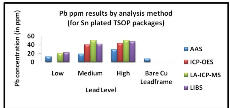
**Table 2.** Comparison of Pb concentration (in ppm) determined by different analytical techniques for Sn plating of TSOP5656 leadframe packages deposited at three different current settings.
